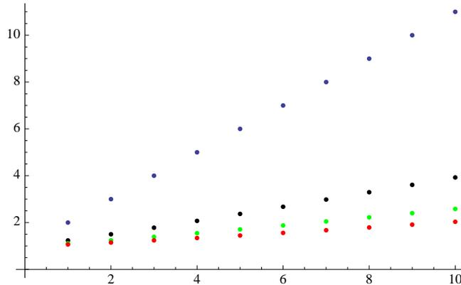
FIGURE 5. Critical value of the ratio of elasticities  $c$  as a function of  $m$ . The top line corresponds to  $\ell = 1$ , the ones below correspond to  $\ell = 2, 3, 4$  (in that order).
