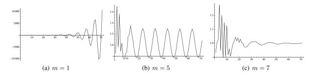
FIGURE 2. As m increases, behaviour changes from unstable to stable.
